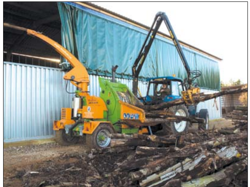
Bill Hannant of King Timber, using AWF's Heizohack HM 10-400-K woodchipper. He is turning 15-inch diameter, 4-metre lengths of poplar, Silver birch and chestnut into chips, sized 25 by 30 mm, with a moisture content of 20 to 25%. They flow straight from the chipper into a newly-finished, purpose-built chip-store, which uses artic lorry sliding-sides to keep the chip aired but not exposed.
